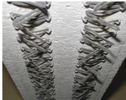
Pinned elements after high temperature cycling
